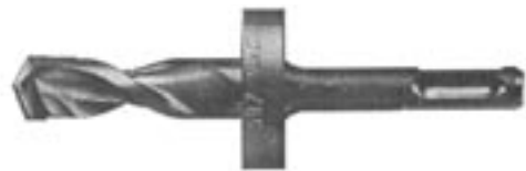
"Stop" or "Collar" drill used in many types of undercut
