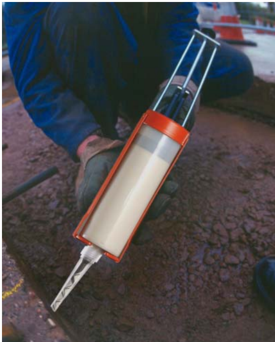
Co-axial cartridge showing two components mixing in the nozzle
